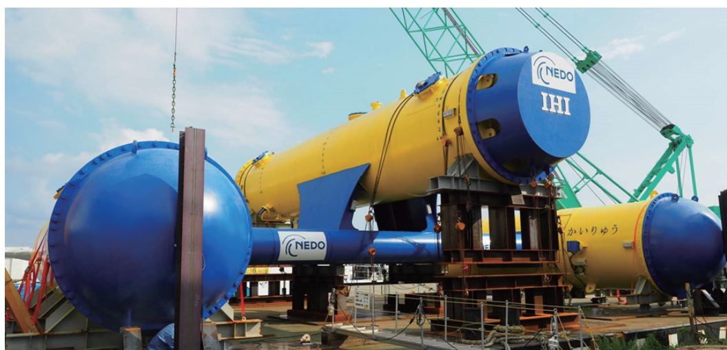
“Kairyu” — 100 kW-class floating type ocean current turbine for demonstration
