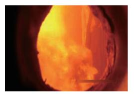
Flame from solo-combustion of oil coke inside the low-volatile fuel burner
