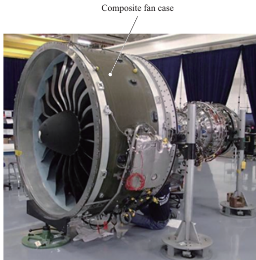
Fig. 12 PW1100G-JM and composite fan case
