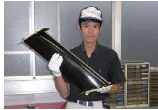
Fig. 13 PW1100G-JM composite SGV
