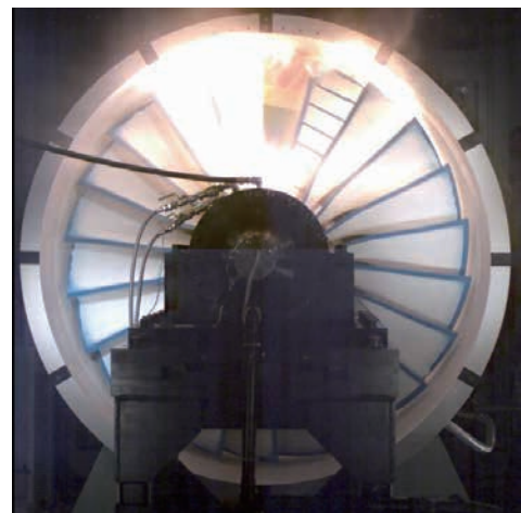
Fig. 8 Containment rig test
