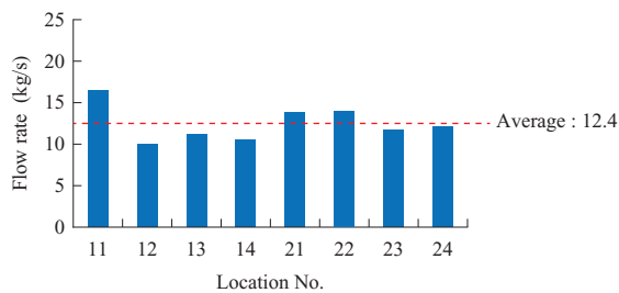
Flow analysis results for the duct with vertical direction plates, and average flow rate distribution at the exit
