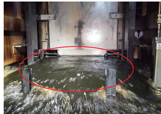
The bump area has become nearly flat Oil flow in the new oil-agitator duct
