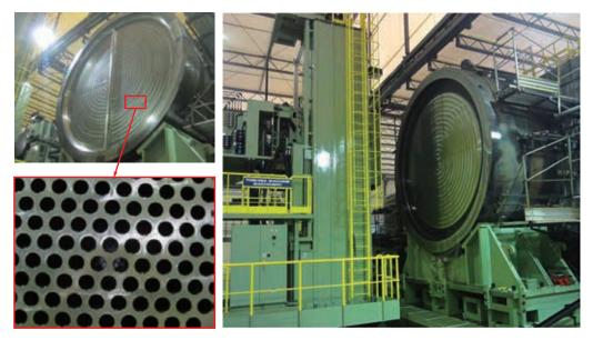
Deep hole-drilling machine for tube sheet BTA (Boring and Trepanning Association)
