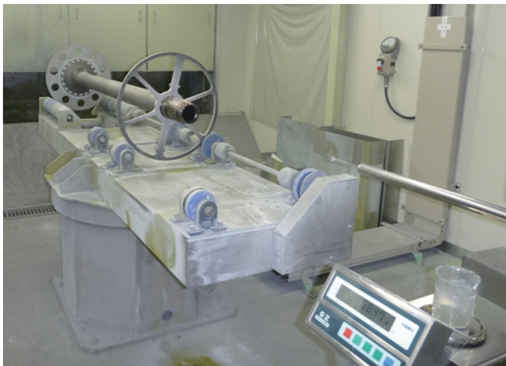
Automated engine shaft coating system
