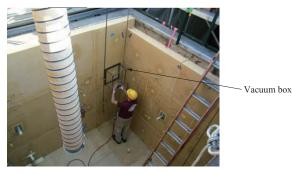
Fig. 7 Vacuum box test applied to the secondary barrier system
