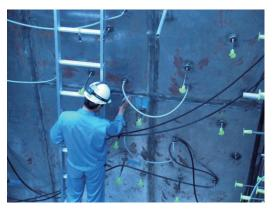
Fig. 8 Helium gas leak test of vapor barrier
