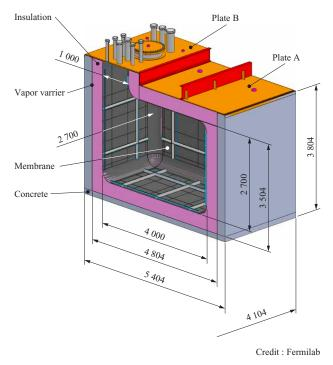
Fig. 2 Liquid argon tank configuration (unit:mm)
