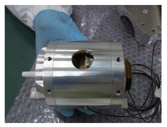
Mock-up chassis including a digital camera for vibration testing
