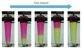
Fig. 3 Plug flow formed in new reactor
