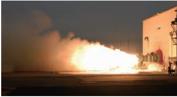
Combustion test of 2nd stage motor ©JAXA
