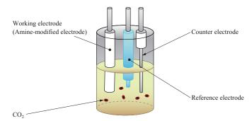
Measurement system for using the amine-modified electrode
