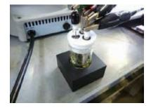
Experiment using amine-modified electrode
