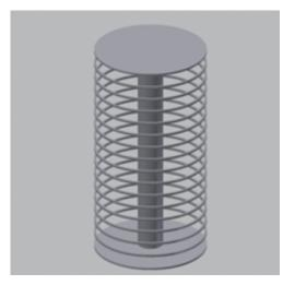
Fig. 9 Small-diameter-cylinder-type ODR satellite
