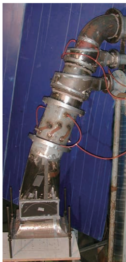
(a) Pulverized-coal pipe (burner inlet)
