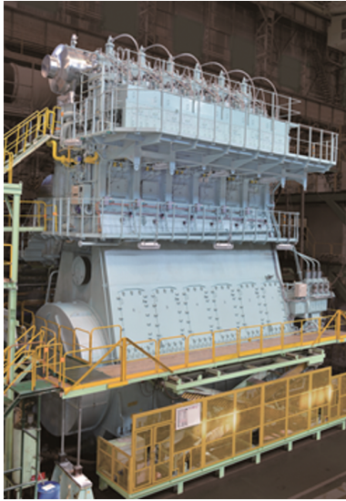
Fig. 1 2 stroke test engine in IPS (6X72DF)
