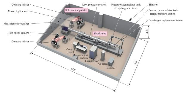
Overall view of the shock tube for blast injury research (unit : m)
