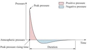
Shock wave pressure waveform
