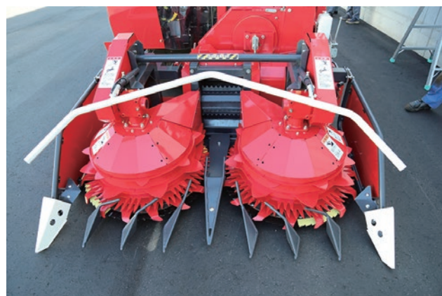
Rotary header-type harvesting unit
