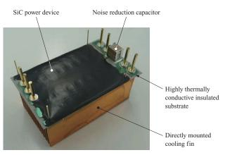
Fig. 10 Prototype of SiC power module
