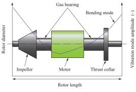
Fig. 6 Illustration of critical speed analysis
