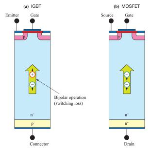
Fig. 7 Schematic cross sectional view of IGBT and MOSFET structures
