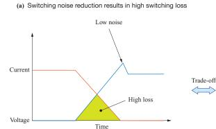
Fig. 9 Trade-off of switching characteristics
