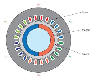
Fig. 1 Schematic cross sectional view of the high speed motor
