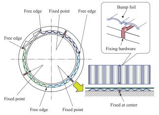
Fig. 5 Schematic cross sectional view of foil-type dynamic radial gas bearing designed to have bump foil with three segmental structure
