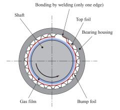
Fig. 4 Schematic cross sectional view of foil-type dynamic radial gas bearing
