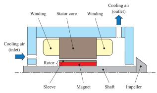
Fig. 2 Schematic cross sectional view of high speed rotating machinery
