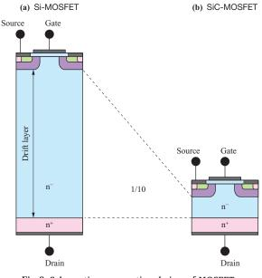
Fig. 8 Schematic cross sectional view of MOSFETs
