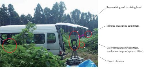
Main unit of measuring equipment (mounted on vehicle)
