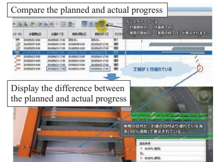
(c) Check on the difference between the planned and actual progress
