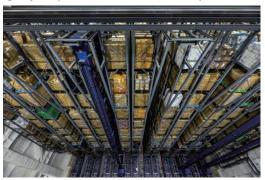
Exterior view of seismic isolation AS/RS at downward angle
