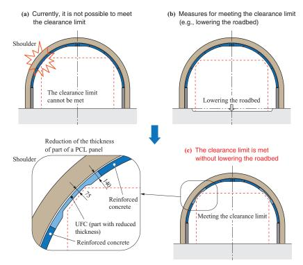
Schematic diagram of partially thin PCL panel (unit: mm)
