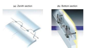
Detailed view of connection of PCL panel
