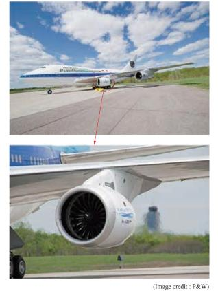
Fig. 4 PW1100G-JM first engine ground test and FTB test<sup>(1)</sup>
