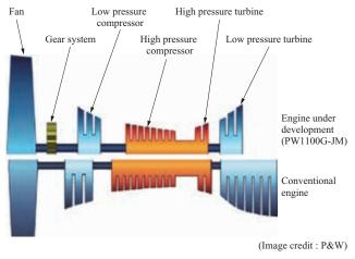
Fig. 5 Comparison of PW1100G-JM and conventional engine configurations <sup>(1)</sup>
