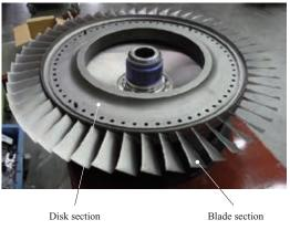
Fig. 9 Low pressure compressor stage-2 IBR
