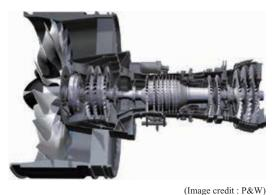
Fig. 2 PW1100G-JM cutaway view<sup>(1)</sup>
