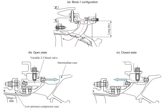
Fig. 10 Variable 2.5 bleed valve cross-section
