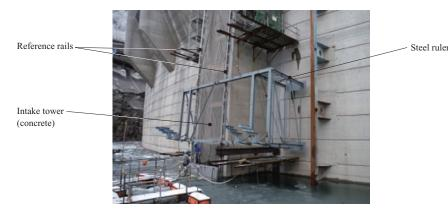
Fig. 9 Survey using the reference rail
