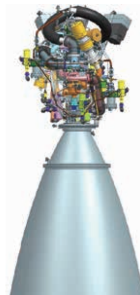
Expander cycle methane engine with thrust class of 3 tons ©JAXA
