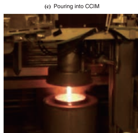
Fig. 4 Appearance of a cold crucible induction melter (CCIM)
