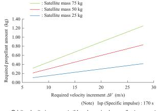
Orbit velocity increment  $\Delta V$  and required propellant amount when using low-cost green propellant thruster
