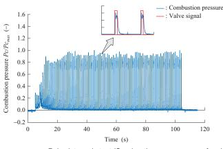
Pulse jet mode test (Combustion pressure waveform)
