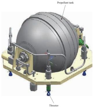
Schematic diagram of propulsion unit
