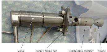
Schematic diagram of green propellant thruster for very small satellites
