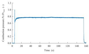
Continuous jet mode test (Combustion pressure waveform)
