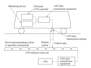
Fig. 5 ATO Data Transmission Equipment Configuration
