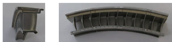
Fig. 13 Sintered prototype vanes using new binder
