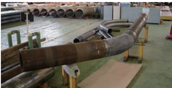
A Ni-based alloy pipe made by high-frequency bending
