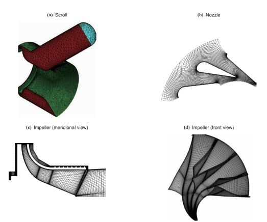
Fig. 4 CFD analysis mesh
