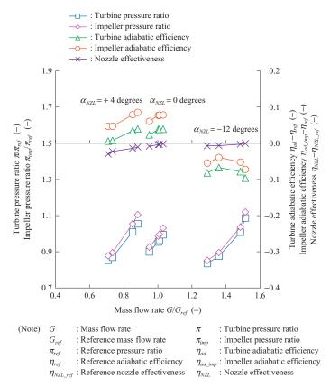
Fig. 8 Overall performance of the turbine, performance of the impeller alone, and nozzle effectiveness
