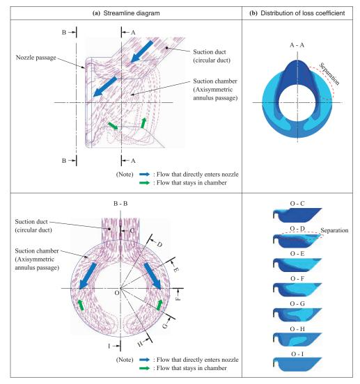
Fig. 6 Flow pattern inside the scroll
