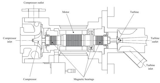
Fig. 12 Cross-section of the turbine-compressor for a 10-kW refrigerator
