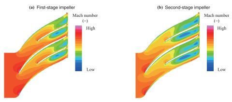
Fig. 24 Distribution of the relative Mach number in the impeller shroud section
