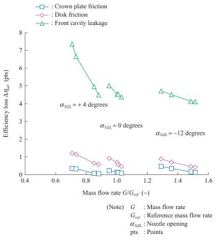
Fig. 10 Impeller disk friction loss and leakage loss
