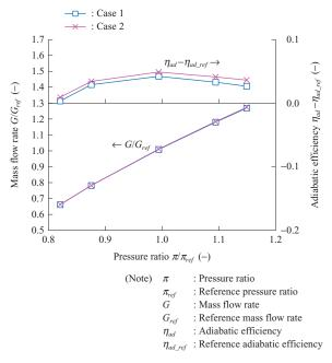
Fig. 14 Predicted overall turbine performance
