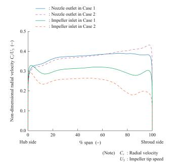
Fig. 16 Spanwise distribution of radial velocity at the nozzle exit and the impeller inlet
