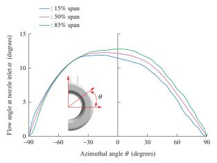
Fig. 7 Circumferential distribution of the flow angle at the nozzle inlet
