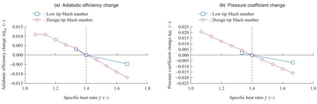
Fig. 22 Influence of the specific heat ratio on the compressor performance
