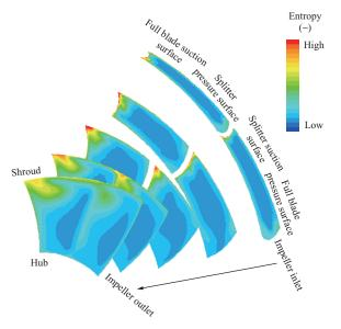
Fig. 11 Distribution of entropy at cross-sectional planes along the flow direction inside the impeller
