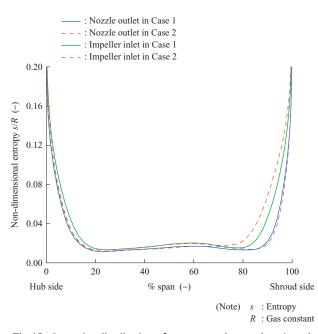
Fig. 15 Spanwise distribution of entropy at the nozzle exit and the impeller inlet
