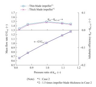
Fig. 19 Predicted overall turbine performance (influence of impeller blade thickness)
