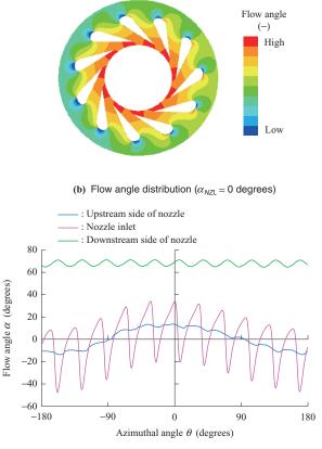
Fig. 9 Distribution of the flow angle in the nozzle mean section
