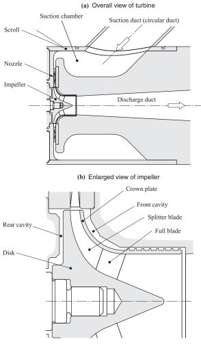
Fig. 3 Configuration of the turbine for a 2-kW research refrigerator
