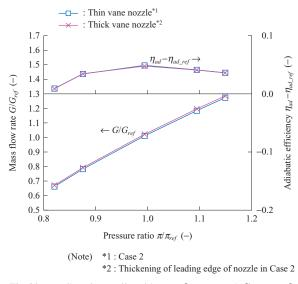
Fig. 20 Predicted overall turbine performance (influence of nozzle vane thickness)
