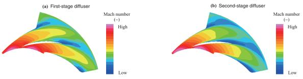
Fig. 25 Distribution of the Mach number in the diffuser mean section
