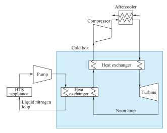
Fig. 1 HTS refrigeration system using a neon turbo-Brayton refrigerator
