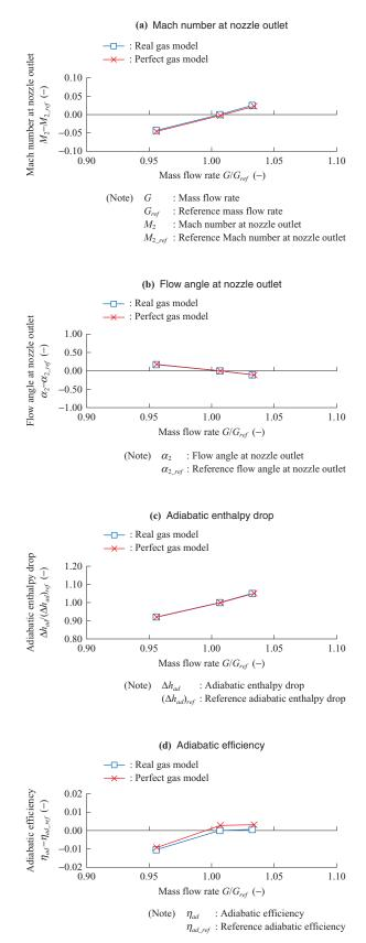
Fig. 5 Comparison of turbine performance predictions using a real gas model and a perfect gas model
