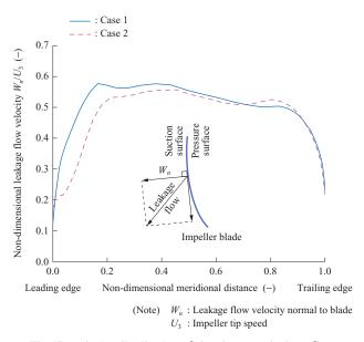
Fig. 17 Velocity distribution of the clearance leakage flow
