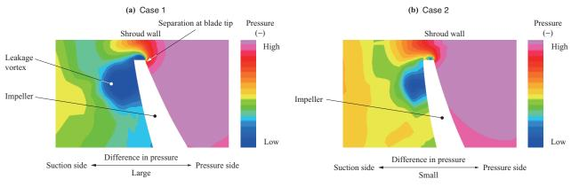
Fig. 18 Distribution of static pressure around the blade tip near the impeller leading edge
