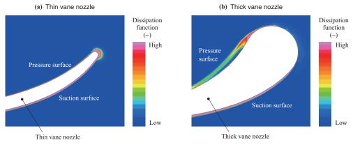
Fig. 21 Distribution of the dissipation function around the vane leading edge in the nozzle mean section
