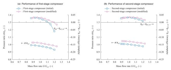
Fig. 23 Predicted overall compressor performance
