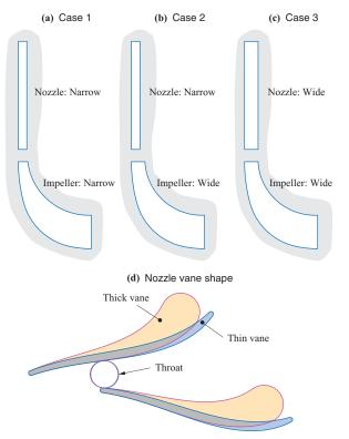
Fig. 13 Impeller shape and nozzle shape
