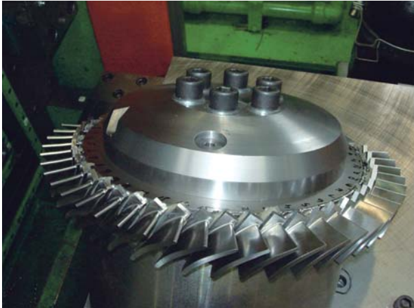
Fig. 9 Demonstrator blisk manufactured by LFW
