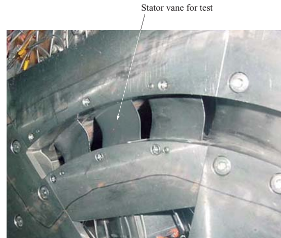
Fig. 14 Annular sector cascade rig
