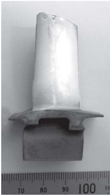
Fig. 25 A turbine blade with YSZ coating by laser-CVD
