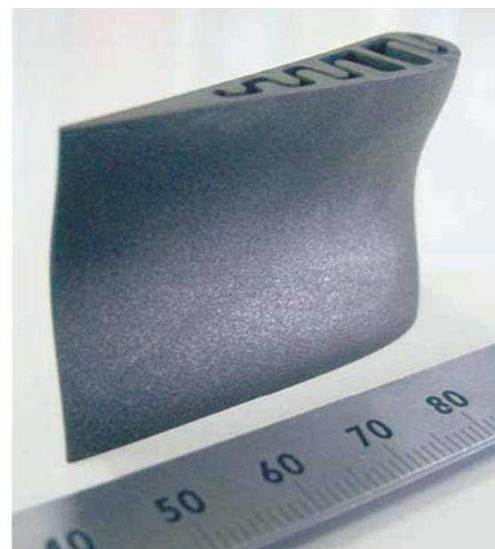
Fig. 15 Photograph of multi-slot cooled vane
