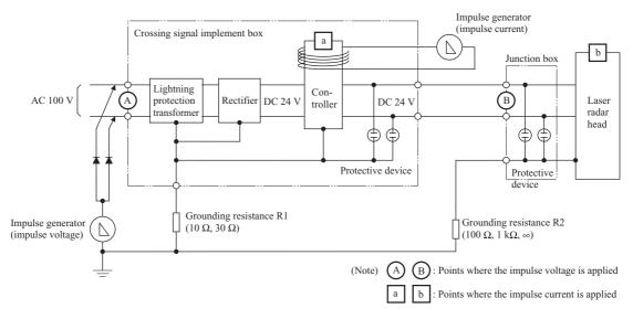
Fig. 5 Circuit of electromagnetic impulse testing
