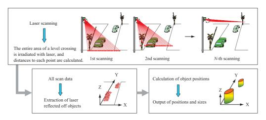
Fig. 3 Object detection method
