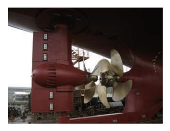
Tandem contra-rotating propeller, rudder propeller (ZP-41RP)
