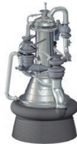
Fig. 1 Illustration of LE-X engine exterior
