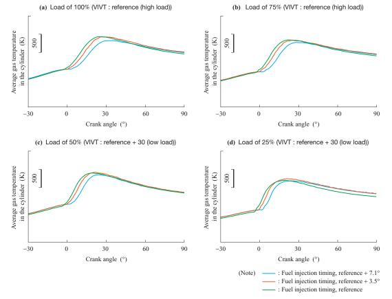
Fig. 9 Comparison of mean in-cylinder gas temperature curves when fuel injection timing changed at each load
