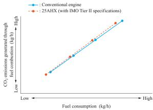
Fig. 6 Relationship between fuel consumption and emissions of  $\rm CO_2$  generated in combustion
