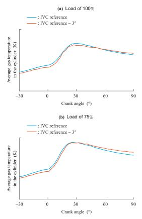
Fig. 12 Comparison of mean in-cylinder gas temperature curves when IVC advanced
