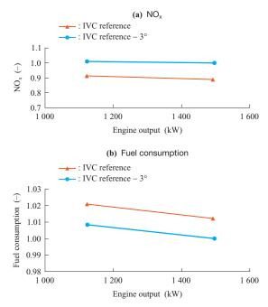
Fig. 13 Changes in  $\ensuremath{\text{NO}_x}$  emissions and fuel consumption when IVC advanced
