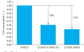
Fig. 17 Comparison of annual fuel consumption among tugboats with different engines
