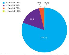
Fig. 16 Percentages of operating time of tugboat in each load range
