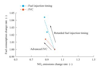
Fig. 14 Changes in  $NO_x$  emissions and fuel consumption due to difference of IVC or injection timing at rated load
