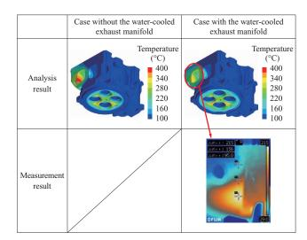
Fig. 18 Comparison of coupled analysis of CFD and FEM with measurement with or without cooling manifold
