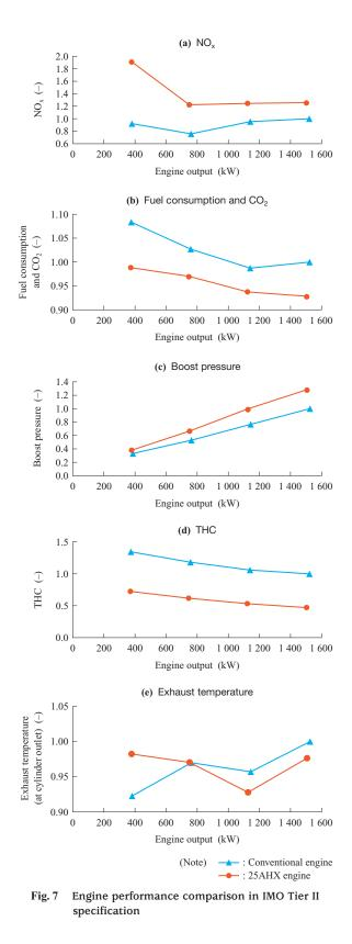
improvements of approximately 7% at the rated output (1 500 kW) and 15% at a load factor of 25%, compared to a conventional engine. When compared with engines that have identical net mean effective pressure (*Pme*) as of 2020, this fuel consumption performance is one of the best in the world.
