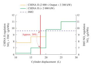
Fig. 8 Comparison of CHINA II exhaust gas emission limits with IMO  $NO_x$  emission limits
