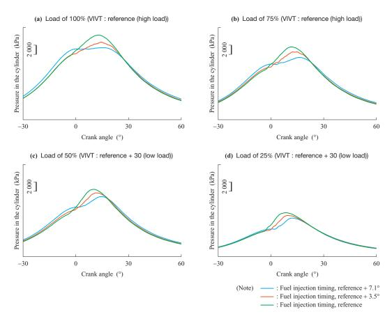
Fig. 10 Comparison of in-cylinder pressure curves when fuel injection timing changed at each load
