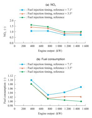
Fig. 11 Changes in  $NO_x$  emissions and fuel consumption due to difference of fuel injection timing
