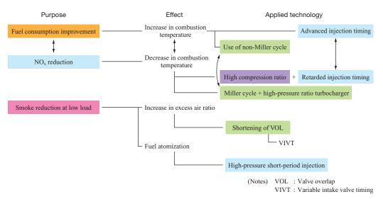
Fig. 4 Technology of NO<sub>x</sub> reduction for AHX series engine
