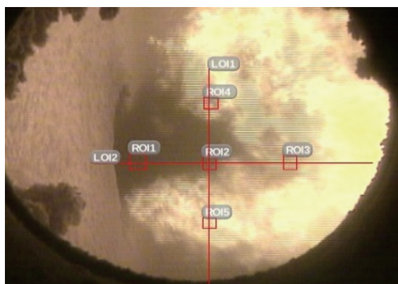
Flame generated during ammonia 20% combustion
