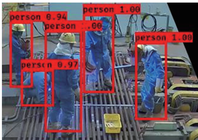
Human detection using ceiling camera (human detection function) (Conducted at the Manufacturing Department, IHI Aioi Works)
