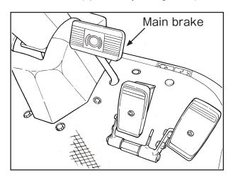
Used to stop the machine. By stepping the pedal, the brake is applied. Safe start device is provided. Be sure to step the safe start device when starting the engine.
