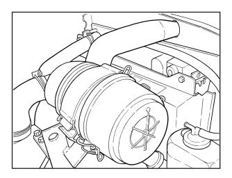
Clean the outer element every 100 hours and replace after cleaning 6 times. When the machine is operated in dusty place, clean the outer element at a shorter interval and replace the element before the specified time limit.
