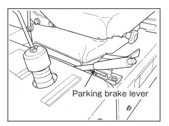
By stepping the main brake and pulling up the rod, the parking brake is applied. To release the brake, step the main brake strongly.
