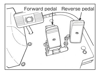
Step the forward pedal to forward the machine and the reverse pedal to reverse it.
