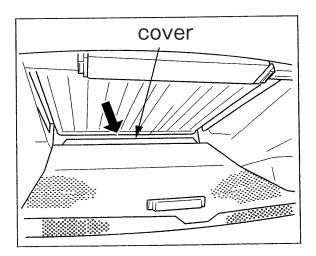
Turf attached to the radiator may cause overheat. Be sure to inspect and clean before and after operation. Inspect during the operation also depending on the operating conditions.
