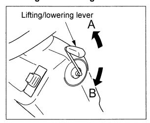
By moving the lifting/lowering lever to the A direction, the mower lifts and by moving the lever to B direction, the mower lowers.
