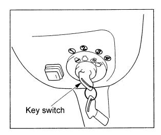
①[OFF]: ····· Position where the engine stops and the key can be inserted or removed.
