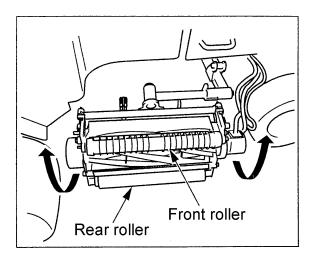
To return to the original position, start the engine and move the lifting/lowering lever to the lifting side. When the reel unit lifted above the ground, move the lifting/lowering lever to the lowering side. Then the mowers return to the position of lapping.
