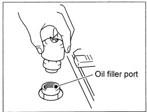
Open the rear cover and front cover. By loosening the bolt fixing the upper cover of the hydraulic tank, the cover can be removed. After supplying the oil, retighten the bolt.
