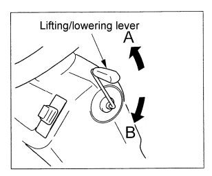
This lever is used to lift or lower the implement. By moving the lever to the A direction, the implement lifts up. By moving the lever to the B direction, the implement lowers.
