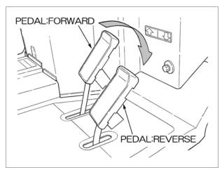
Press forward pedal down to drive the vehicle forward and the reverse pedal to reverse it. No clutch pedal is provided on this machine. Speed is increased or decreased by the amount the pedal is depressed.
