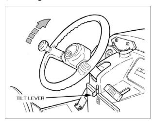
Angle of the steering wheel can be adjusted. Position of the steering wheel can be adjusted by pulling the tilt lever.
