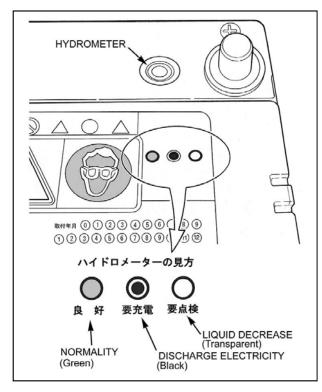
Color which can be seen on the hydrometer indicates the battery condition.
