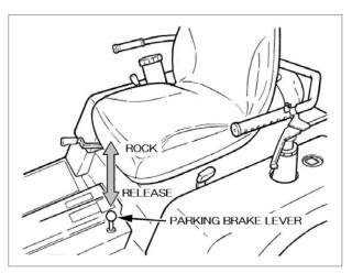
By pressing the brake pedal fully and pulling up the lever, the parking brake is applied.
