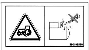
• Do not start the engine by shorting across the starter terminals. Tractor will start in gear if normal circuitry is bypassed. NEVER start the engine while on the ground. Start engine only from operator's seat, with transmission in neutral
