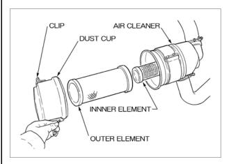
Clean the outer element every 100 hours and replace it after cleaning 6 times. If the operation is carried out in a place subject to excessive dust, clean the air element at a shorter interval. Replace the element about once a year even though the specified interval has not been expired.
