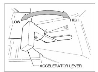
The accelerator lever is used to increase or decrease the engine revolutions.
