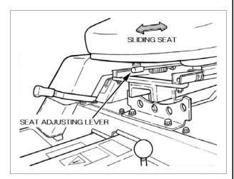
The seat slides forward and backward. Release the seat by movement of the lever. Adjust the seat properly to your operating position.
