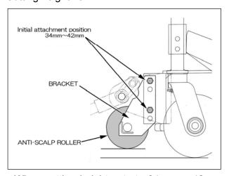
When cutting height sets to 34 mm - 42 mm, please fix with an attached bolt and nut in the hole above a bracket, and the hole above a mower. (Initial attachment position)
