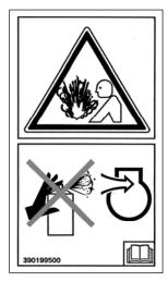
· Do not use ether with the grow plug starting aid or spray. Cause an explosion and fire.
