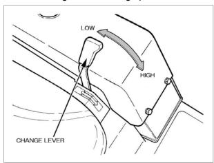
Vehicle speed can be selected from "L" (low speed) (4 WD) and "H" (high speed) (2 WD). By pushing the lever forward, the speed increases and by pushing it rearward, the speed decreases. Keep the lever on the low speed side for usual operation and use the high speed side only when traveling. When changing the speed, stop the vehicle.
