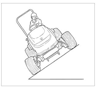
By grasping the seat swing lever above the oil tank, the seat rolls laterally in 2 steps to 12.5 and 15°. Continuous operation along the slope allows safe operation at a comfortable position.
