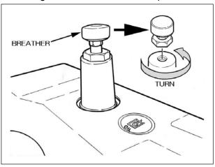
Turn the breather counterclockwise to remove it. After supplying oil, tighten the breather.
