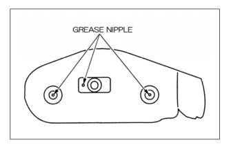
Supply grease to the idler pivot and right and left front gauge wheels every 50 hours.
