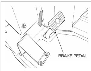
By pressing the brake pedal, brake is applied. A safe starting device is provided. Be sure to press the brake pedal when starting the engine.
