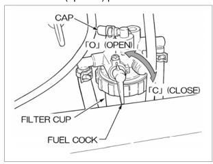
The fuel feed pump of this machine is driven from the cam shaft. After it is operated for cleaning or replacement, remove the cap and discharge the air in the filter cup.
