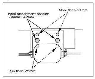
Change the attachment position of an antiscalp roller in three steps according to cutting height.
