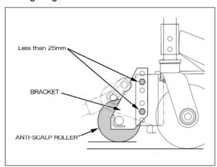
When you set cutting height as 25 mm or less, please fix with an attached bolt nut in the hole of the bracket bottom, and the hole above a mower.
