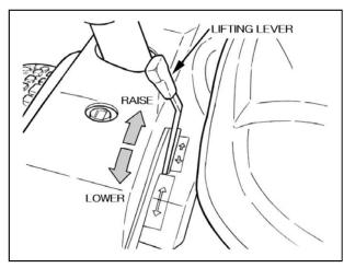
When lifting or lowering the mid mower, push the lifting lever forwards to lower the mower, and push it to the rear to lift the mower. When you leave your hand from the lever, it automatically returns to the neutral position.
