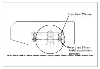
When cutting height is 34 mm or more, please fix a bracket in a lower position. (Initial attachment position)
