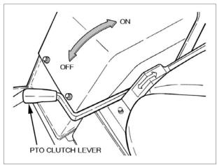
By moving the PTO clutch lever to "ON", the blades rotate. By moving the PTO clutch lever to "OFF", the clutch is disengaged and the blade stops rotating.
