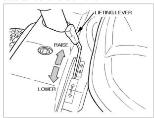
By pushing down the lever rearward, the mower rises. When you release your hand from the lever, it automatically returns to the neutral position. By setting the lever to the lowering position, the lever is held at the lowered position and the mower becomes free to float over undulating ground.
